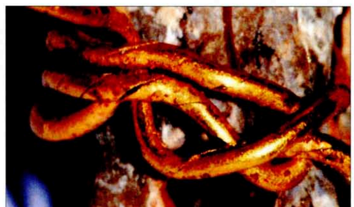
Fig. 8: The gold wire was made by twisting a thin tape of pure gold.
